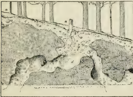
SECTION OF PAINT MINE IN A BED OF IRON ORE, MISSOURI. DEPTH OF EXCAVATIONS ABOUT 20 FT. (HOLMES)
